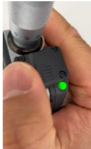
Flashing green (connection complete)
