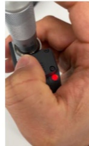
Flashing red (connection failure)
